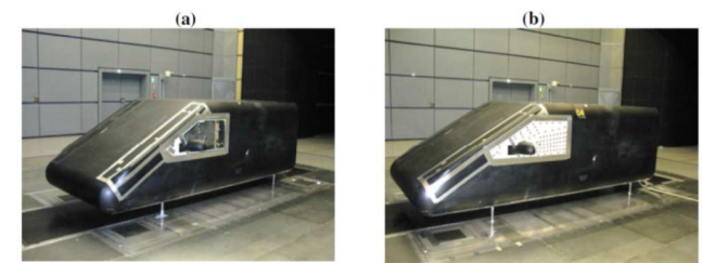
Figure 38. Wind-tunnel test: (a) glass module, (b) sensor module
