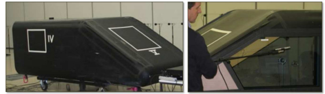
Figure 29. Noise Reduction (NR) measurements performed on several patches around the SAE body.
